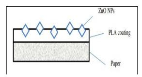
**Gambar 2.** Schematic illustration and structure of food packaging as paper coating from PLA-ZnO
