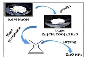
Gambar 1. Synthesis of ZnO Nanoparticles
