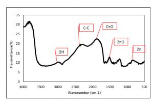
Gambar 3. Spectrum of FTIR ZnO Nanoparticle
